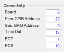
Adjust the cannel setting of your GPIB device. The address is according to device default specifications of CMT is (primary address CMT = 25).
